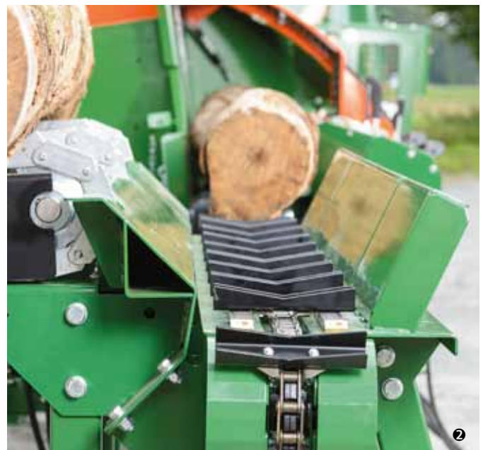
Constant supply thanks to the log conveying system, comprising 1 cross conveyor and 2 chain conveyor.
