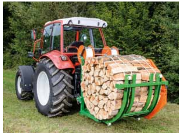
The bundling device as ideal addition to all wood splitters: Bundles half-metre and metre-long logs with composite band.
