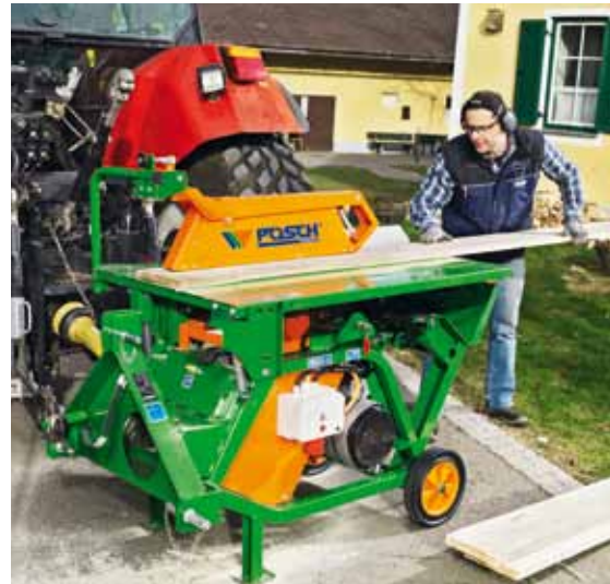
The table tilting saw enables precise cutting in the lengthwise cutting position on the tractor.
