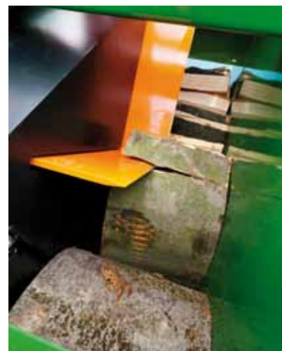
Splitting with adjustable billet size with the X-shaped splitting knife.
