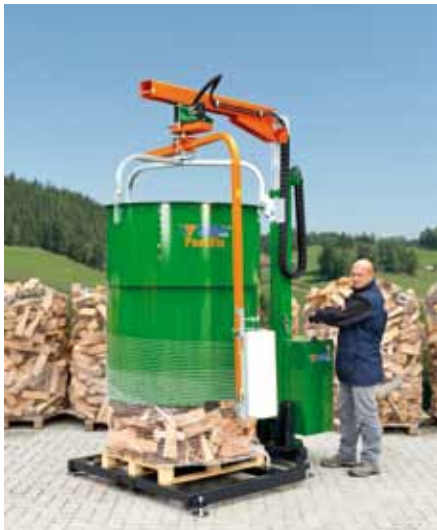
The rotary arm securely wraps the round bale mesh around the filling drum and the billets.
