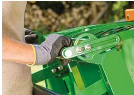
Safety handle with ergonomic height adjustment
