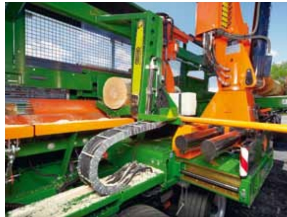
Maximum cutting and splitting power guaranteed. At the core of the SpaltFix K-550, there is a SuperCut chain saw with 75 cm and stepless, hydraulic cutting length adjustment.
