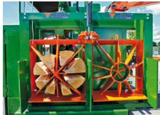
With the hydraulically adjustable frame knife, the SpaltFix K-550 produces up to 18 billets per work cycle (optional with SplitControl for splitting in the middle).
