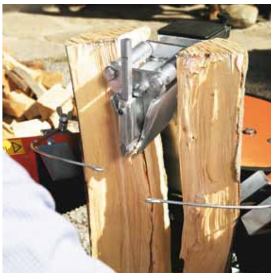
The push-on splitting knife with rollers does the job quickly and thoroughly.
