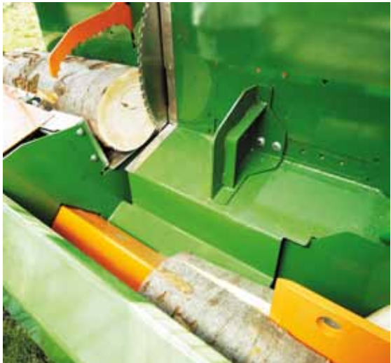
The core of the SpaltFix S-280 with timber downholder, saw blade, adjustable timber stop and splitting knife.
