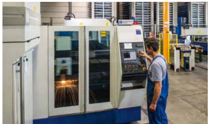
Precision ensured by the sheet metal cutting process applied to each part in the CNC-controlled laser cutting facility.
