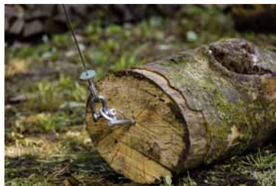
The rope winch with standard prick punch pulls logs to the HydroCombi even on rough terrain.
