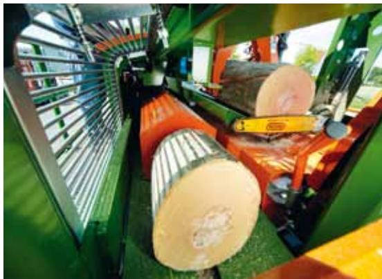
The OptiSplit system automatically adjusts the splitting stroke to the billet length and ensures a higher working speed.
