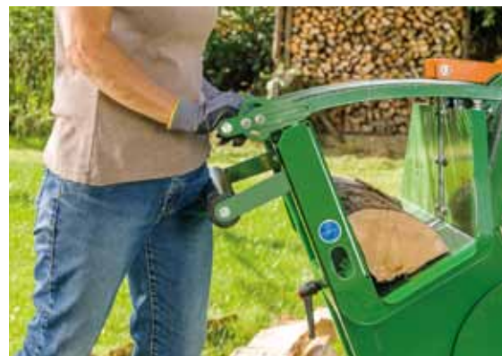
The hip roller in action for effortless cutting
