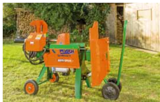
Model with standard timber support table in transport position with transport aid.
