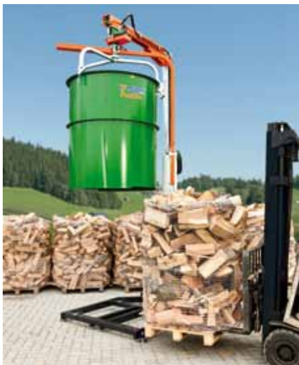
As soon as the filling drum has been pulled up all the way, the mesh is severed and the pack of billets is carted away.
