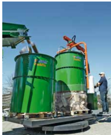
As filling and packing up are done at the same time, the tilting table saves you a lot of time.
